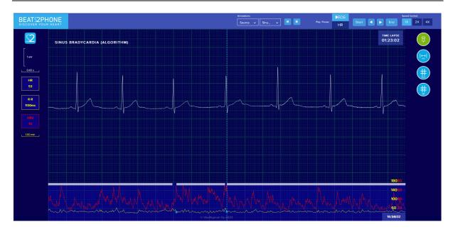
On the left of the screen, you can see the scale of the measurement view. Two squares vertically are 1.00 millivolts, and two squares horizontally are 0.400 seconds. The horizontal scale can be zoomed in and out with the mouse scroll wheel. You can reset the scale by clicking the Beat2Phone logo on the left. In addition, the heart rate is displayed on the left.
